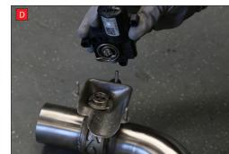
A) After you have removed O.E exhaust you will need to swap the valve motor to the Scorpion exhaust. Remove the 3 nuts (keep them safe, as you will need them to bolt the electronic valve motor to your Scorpion Exhaust).
